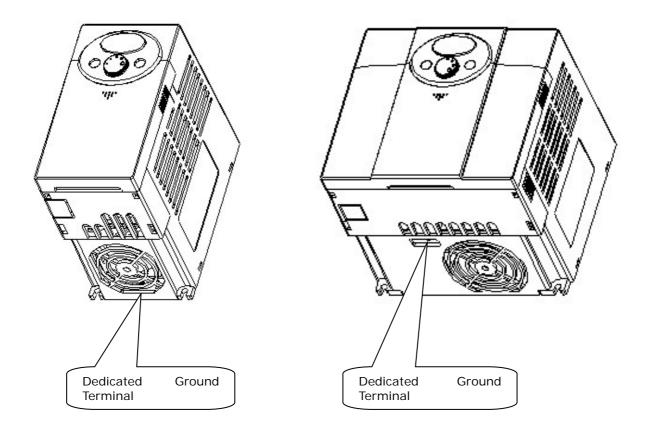
Note: Remove front and bottom cover before starting grounding. Caution: Follow the specifications below when grounding the inverter.
